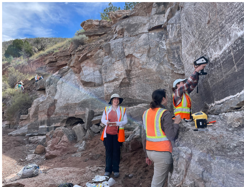
Zoë Havlena (NMT) collecting X-ray fluorescence data from gypsum in the Upper Yeso Formation with Amy McAdam (left) and Christine Knudson (middle), NASA Goddard Space Flight Center during the GIFT program.
