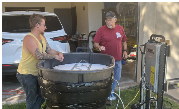
Jon Davis and Devlin Willingham test the hot water bath setup for decontaminating cave gear.
