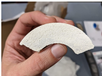
Photo courtesy of Emma Piercey. A ceramic filter used in leaching experiments for Emma Piercey's water filter research.
