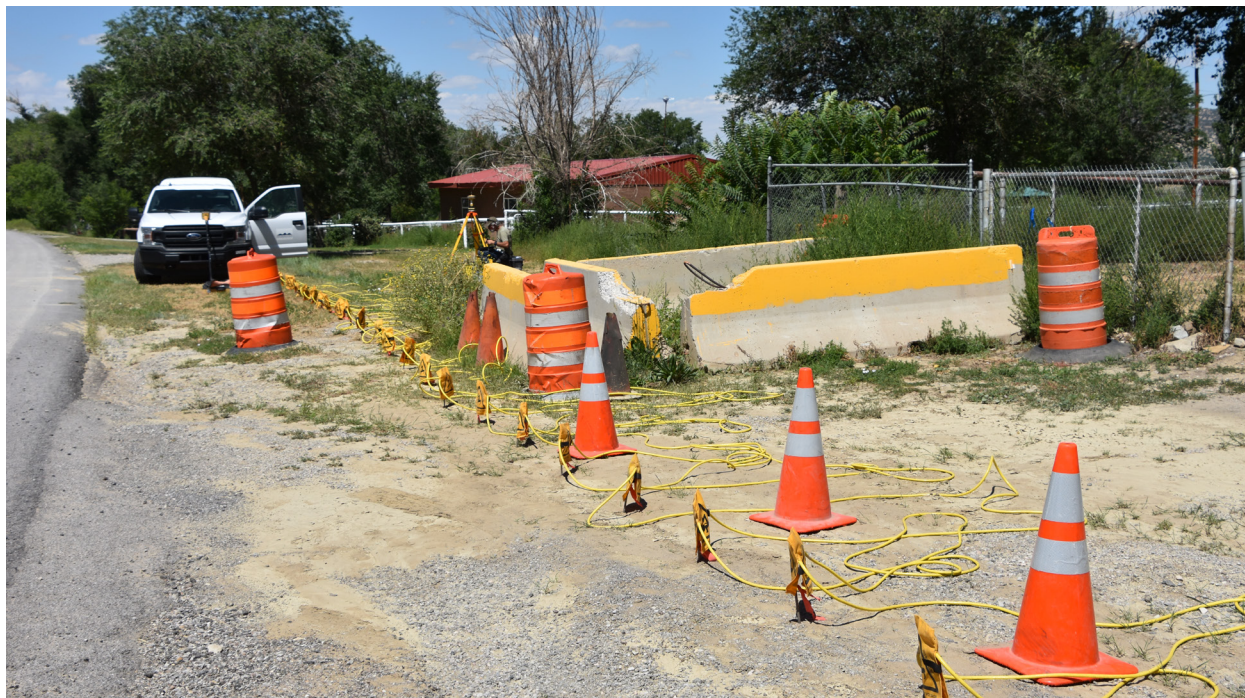
NCKRI photo by George Veni. The electrodes and cable for electrical resistivity line SM2 (see profile above) 2 m south of the San Mateo sinkhole.
