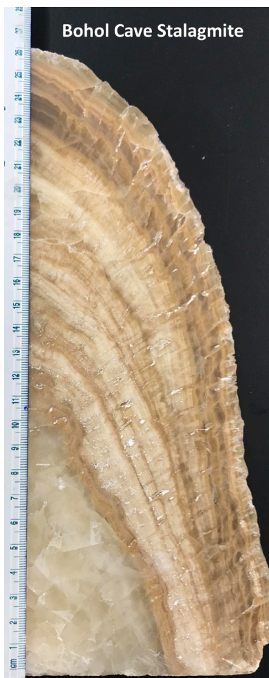
Photo courtesy of Dr. Daniel Ibarra. Polished cross section of a stalagmite from a cave on Bohol Island, Philippines. Analysis of the growth layers will reveal information about paleoclimatic conditions in the Philippines.
