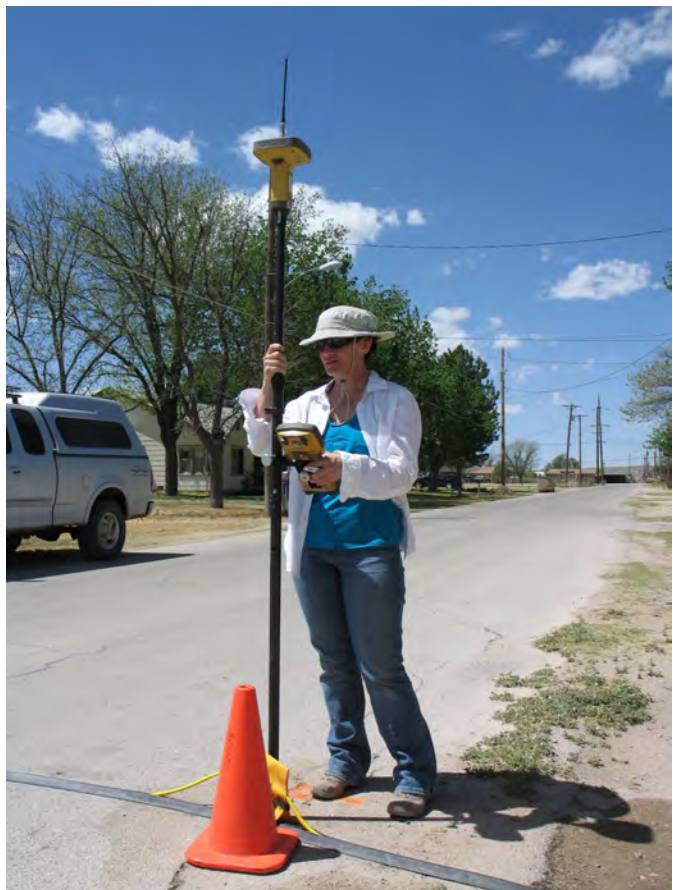
Figure 4. NCKRI's Education Director, Dianne Gillespie, collecting centimeter-precision three-dimensional location coordinates for each electrode. Photo by George Veni.
