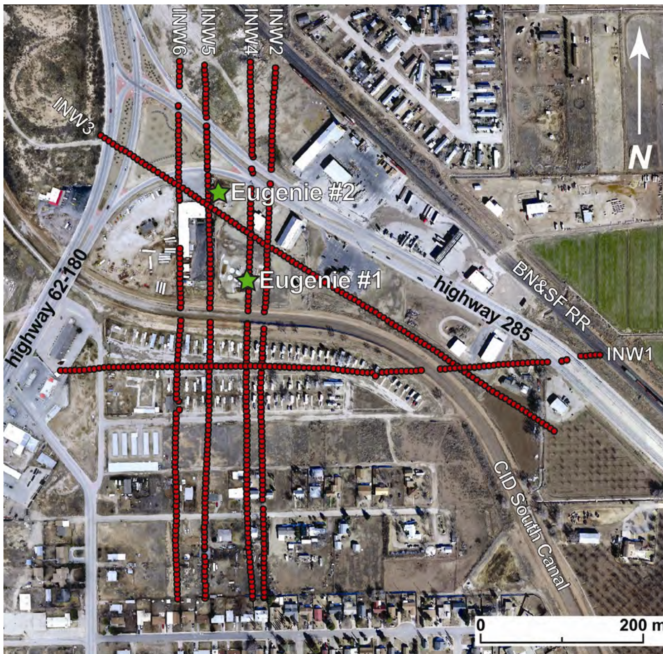
Figure 2. Aerial photo of I&W brine well facility and surrounding area, Carlsbad, New Mexico. Locations of Eugenie #1 and Eugenie #2 wells are shown by green stars. Electrical resistivity survey lines INW 1 through 6 are indicated by red dotted lines. Each dot represents one of the electrodes in the survey line (electrodes lacking GPS coordinates are not shown).
